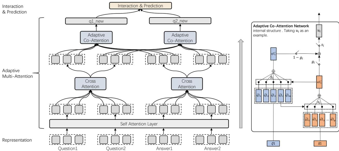
**Figure 2: The overall view of our model. The left part is the main framework of this work. The right part is the detailed structure of the adaptive co-attention network. The thick arrow indicates that information flows from bottom to top.**
